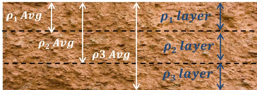
Barnes Method to calculate “Soil Layer Resistivity”
